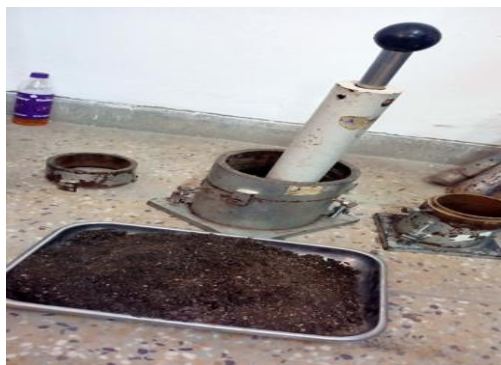
Fig -2: Compaction Rammer and Mould
