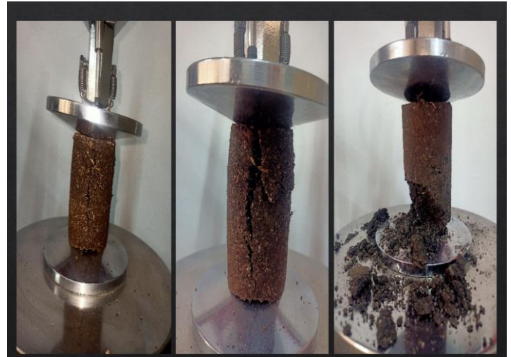
Fig -4: Failure of sample of soil and soil with stabilizer due to unconfined compressive strength
