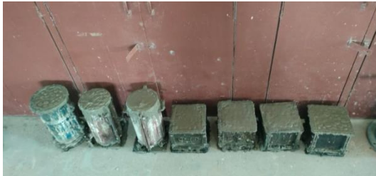
Figure 8.sample of cube Casting
