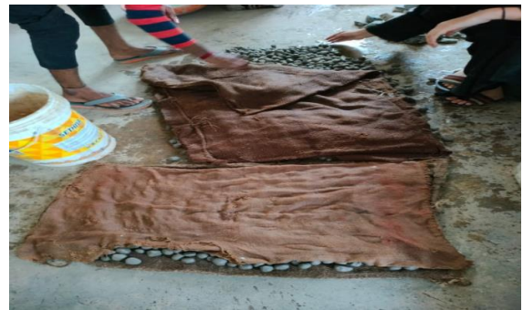
Figure 6. Curing of fly ash aggregate
