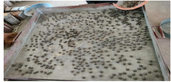
Figure 5. Drying of fly ash aggregate
