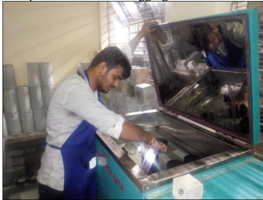
Fig. 1: Placing compacted sample in 60°C water bath
