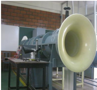
Fig 2a: Pictorial Representation of Axial Ducted Fan Set Up
