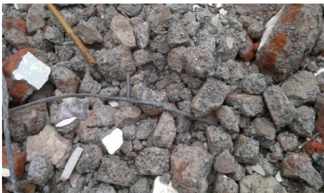
Figure 1: Concrete debris collected from site
