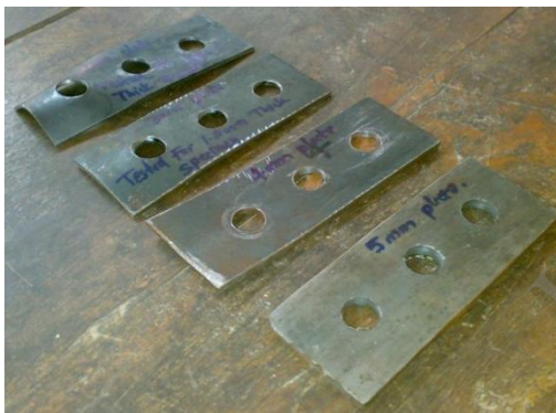
Buckling of Stiffener/Packing plate used 1.5mm Thick Sample Specimen
