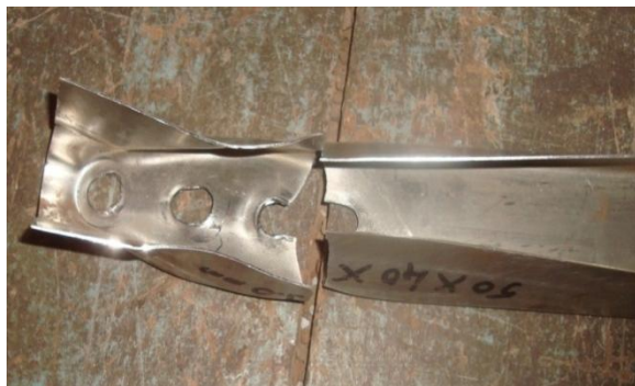
Bearing + Rupture Failure Observed
