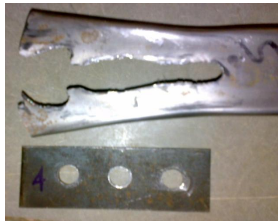
Vertical Shear Failure of 1.5mm Thick Sample Specimen using 4mm thick Stiffener/packing plate
