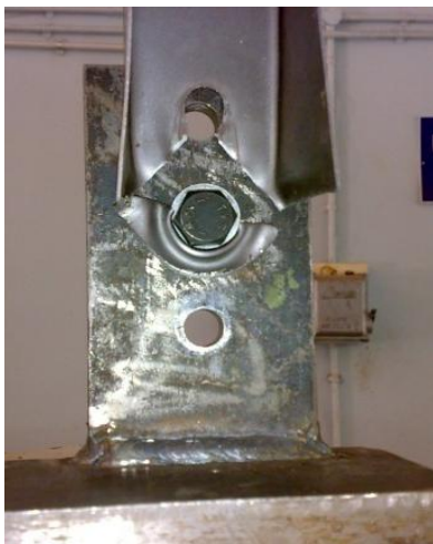
Bearing + Shear Failure Observed for 1.5mm thick specimen sample with single bolted connection
