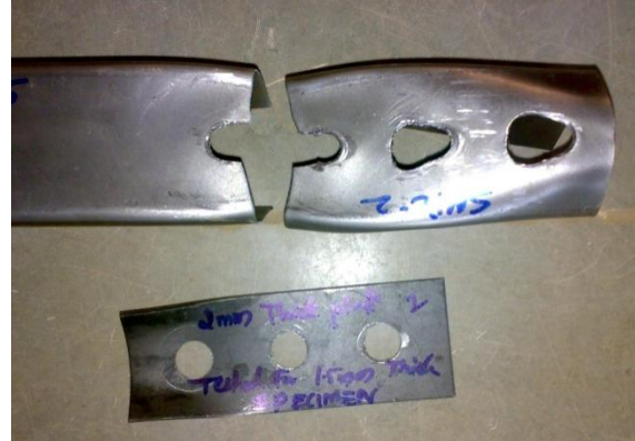
Bearing + Rupture Failure Observed With 2mm Thick Packing Plate for 1.2, and 1.5mm thick specimen sample
