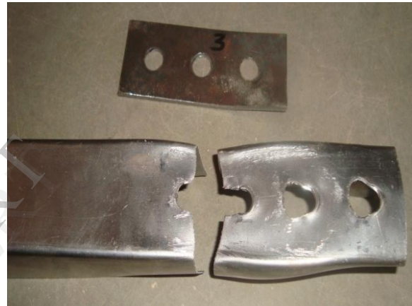
Bearing + Rupture Failure Observed With 3mm Thick Packing Plate for 1.2, and 1.5mm thick specimen sample
