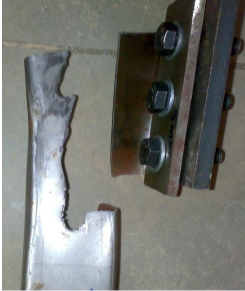
Block Shear Failure of 1.5mm Thick Sample Specimen using 5mm thick Stiffener/packing plate
