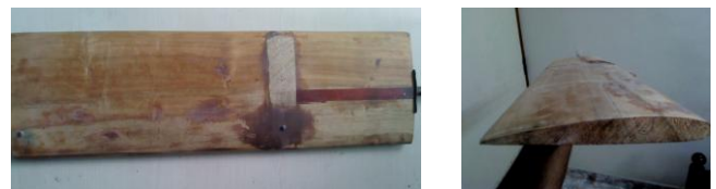
Fig 2.1 Top view and cross-section of wing section NACA 2412
