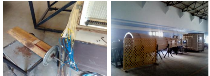
Fig 2.5 Wing section before install into the windtunnel
