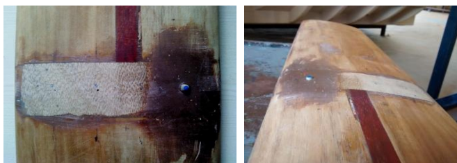
Fig 2.7 Attachment of dimple on the surface of wing section
