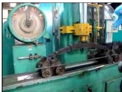
Figure 12 :Fatigue Testing Machine (leaf spring at initial stage)
