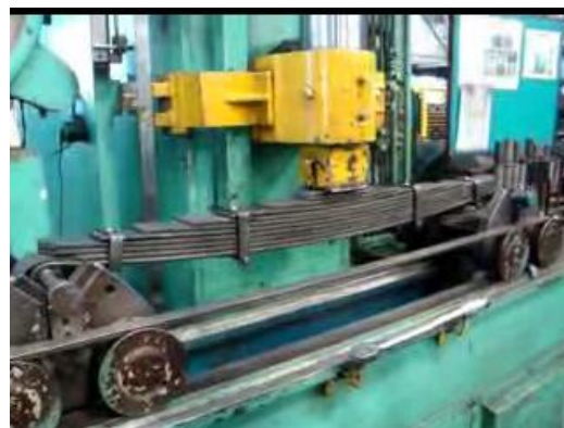
Figure 13: Fatigue Testing Machine (leaf spring at load applied stage)
