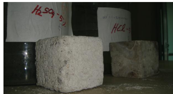
Figure : 4 – Test specimens after immersed in different solutions
