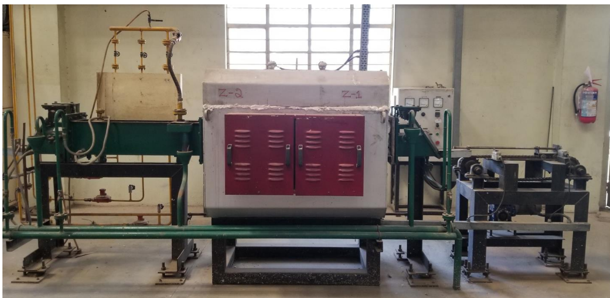
Fig. 1. Furnace used for reduction of coarse blue dust.
