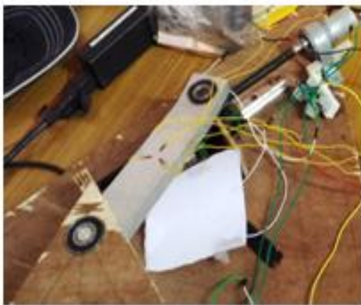
Fig.4. Strain Gauge Rosette installed on non-planar link
