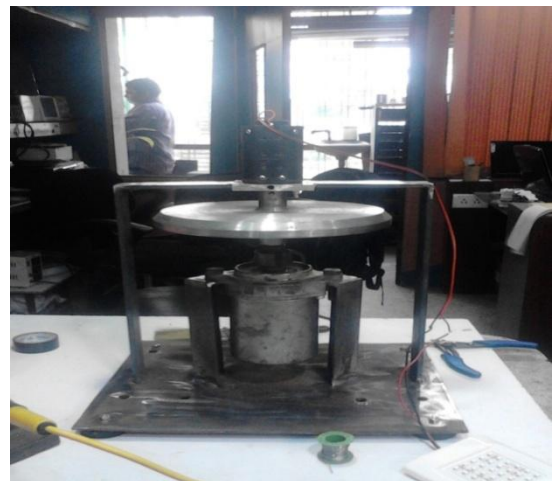
Fig 3: set up of flywheel with motor and generator.
