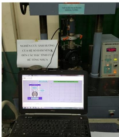
Figure 3.3: Marshall test and stability determination in accordance with ASTM 6927
