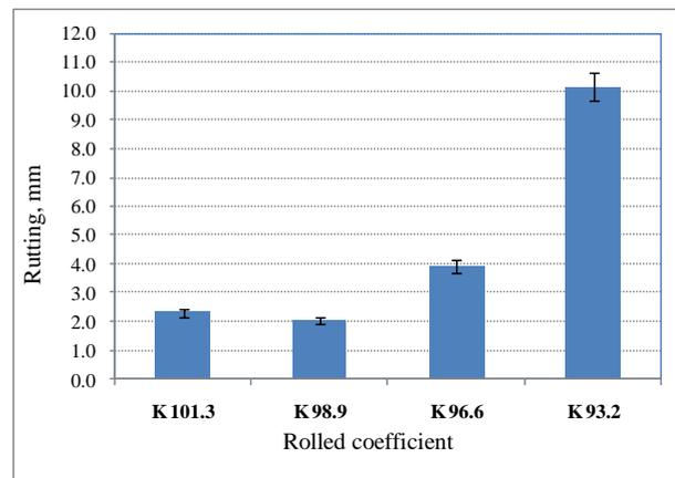
Figure 4.2: Effect of compaction coefficient to splitting R and rutting depth
