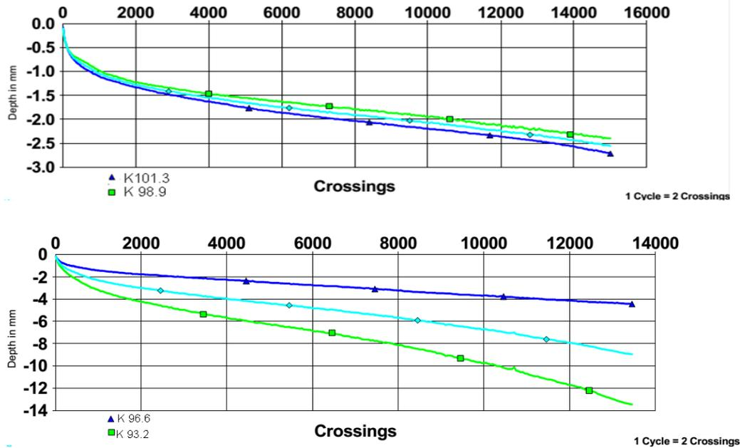
Figure 4.3: Excess distortion accumulation in rutting test of AC samples
