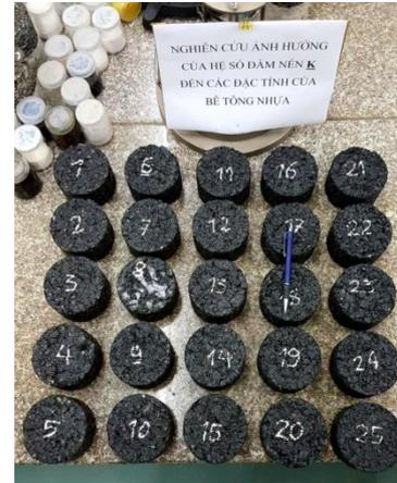
Figure 3.1: Aggregate component of hot mix asphalt BTNC12.5 and samples prepared by rotary rammer
