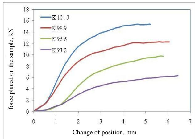
Figure 5.1: Effect of compaction coefficient to AC's technical and mechanical characteristics
