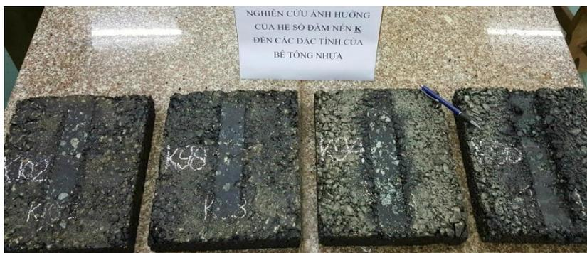
Figure 4.4: Image of AC sample after rutting test
