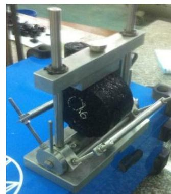
Figure 3.2: Rutting and splitting tensile strength test
