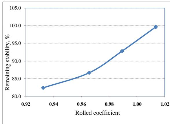
Figure 4.5: Effect of compaction coefficient to AC's moisture resistance
