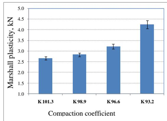
Figure 4.1: Effects of compaction coefficient on Marshall indexes of asphalt concrete
