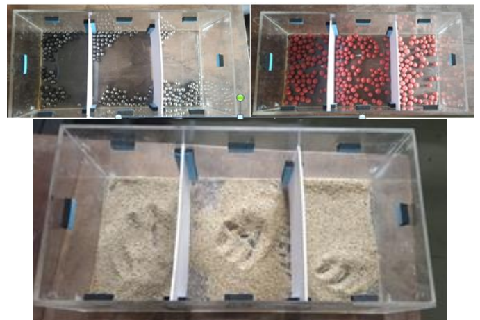
Fig.14. Particles in partitioned damper cavity
