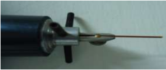
Fig 4.3: Electrode diameter of 0.9mm
