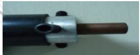
Fig 4.2: Electrode diameter of 8mm
