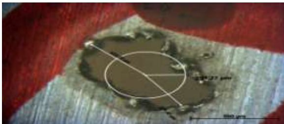
Fig 5.10 (b) Bottom side of micro hole using 0.9 mm copper tool
