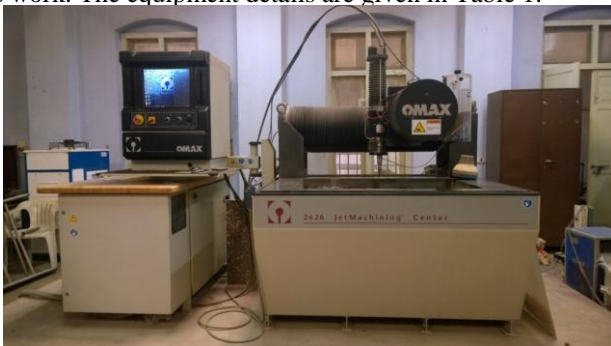
Fig. 2. Photograph of the AWJM setup at Anna University
