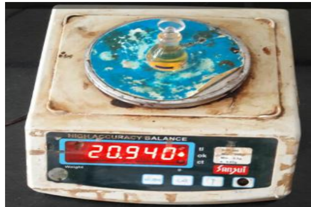
Fig.No.2.Set Up For Density Measurement of Fuel with Magnetization
