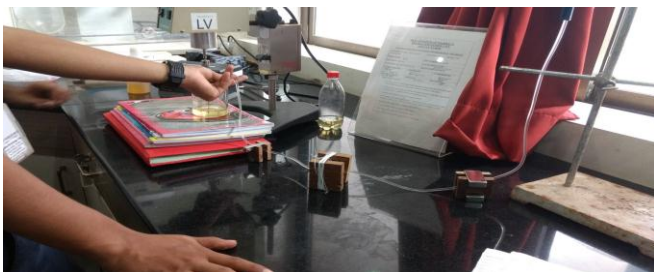
Fig.No.1.Set Up For Viscosity Measurement of Fuel with Magnetization. a.
