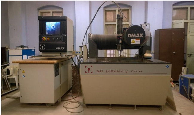
Fig 9: Photograph of AWJ machining setup facility
