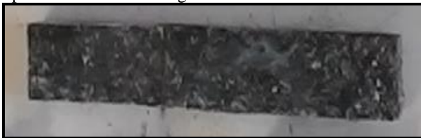
Fig. 1: Flexural test specimen.
