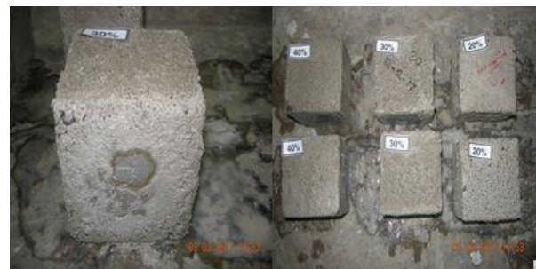
Fig 3: Deteriorated cubes on 3rd day after immersion
