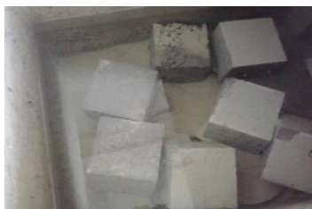
Fig. 2: Curing of Concrete
