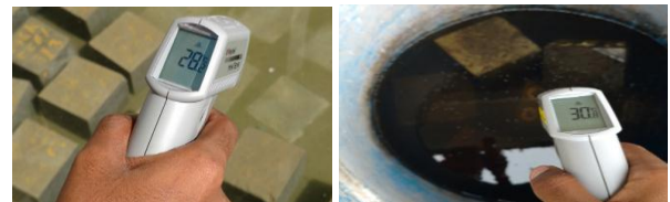
Figure 3: Infrared Thermometer for measuring Surface Temperature
