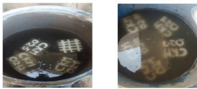
Figure 2: WCO added cubes in Curing medium
