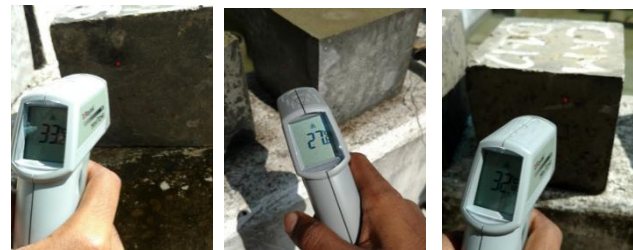
Figure 5: Measurement of Surface Temperature of Concrete Cubes Using Infrared Thermometer
