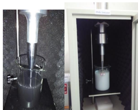
Fig. 2. Probe sonicator used for preparation of CuO and Alumina nanofluid
