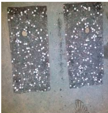
Fig .10. Concrete with 20% replacement of EPS beads
