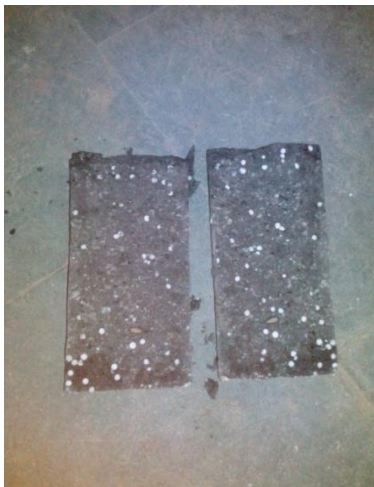
Fig .9. Concrete with 10% replacement of EPS beads
