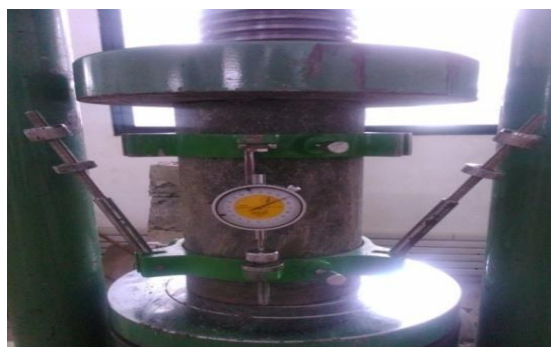
Fig 3.4.2 Elastic modulus test
