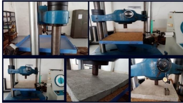
Fig 3.4.4 Load test on slab
