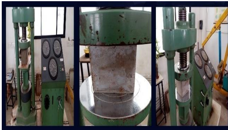
Fig 3.4.1 Compression test on cube
