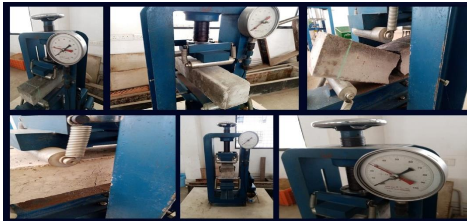
Fig 4.4.3 Flexural strength test on beam
