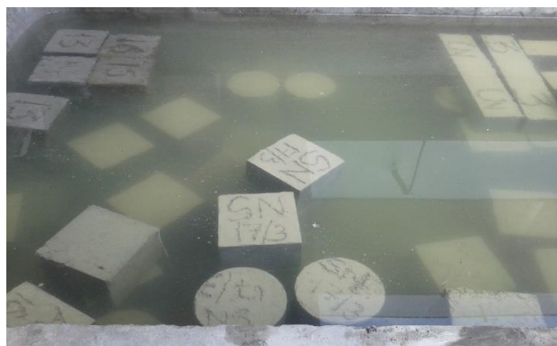
Fig 3.2.2 Curing of specimen
