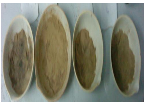
Bagasse Ash after heating in furnace for 1hr; 2hr;3hr and 4hr resp.,
