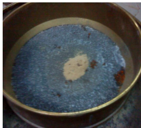
Bagasse Ash passing 150micron sieve
