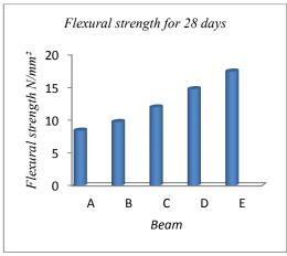
A = Reinforced concrete normal beam
