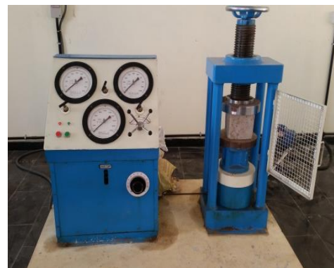
Figure 5. Compressive strength testing.
