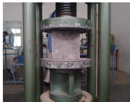
Figure 4.2: Compressive Strength Test
