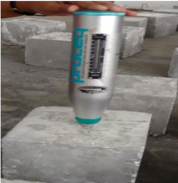
Figure 4.1.1: Rebound Hammer Test
