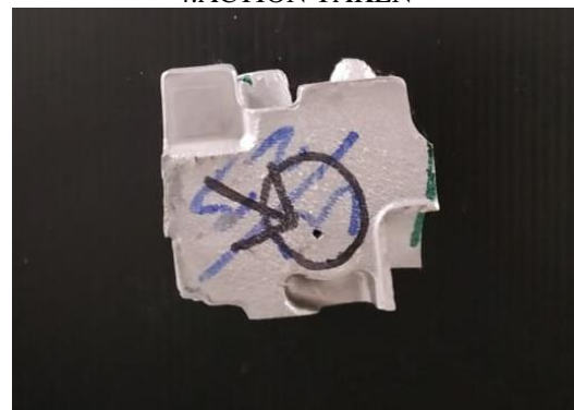
Fig 6: Blow-hole defect cut piece.
