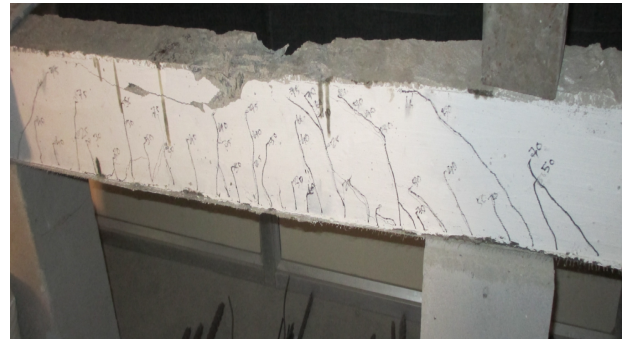
Fig:5.10: Tested of control beam
