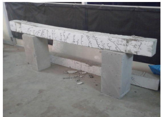
Fig.5.18: Tested GFRP strengthened beam -case 2
