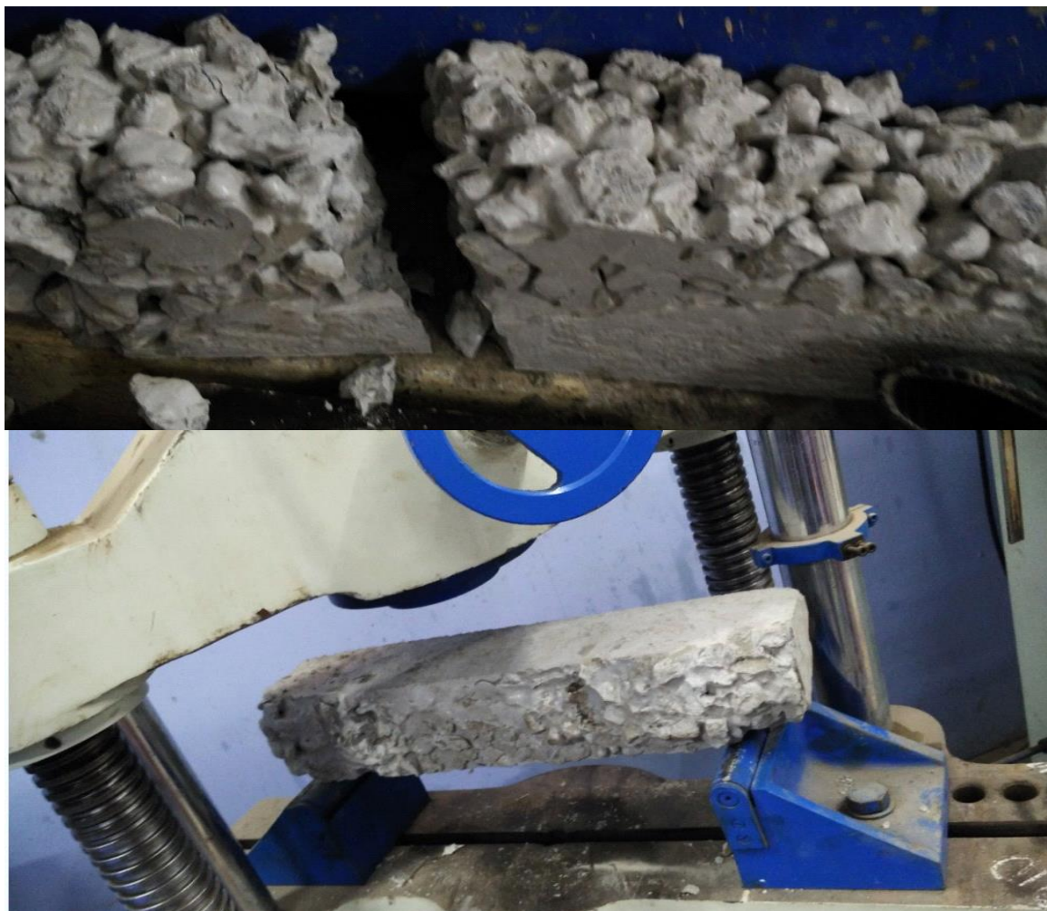
Fig 3.16 Flexural Testing made on loading frame
