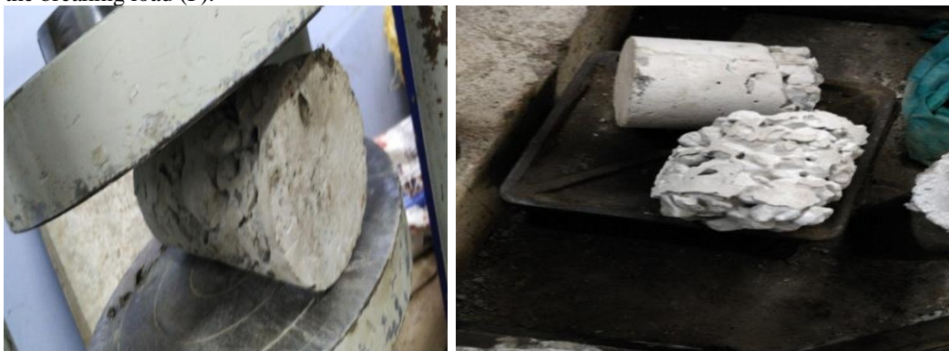
Fig 3.18 Split tensile strength test
