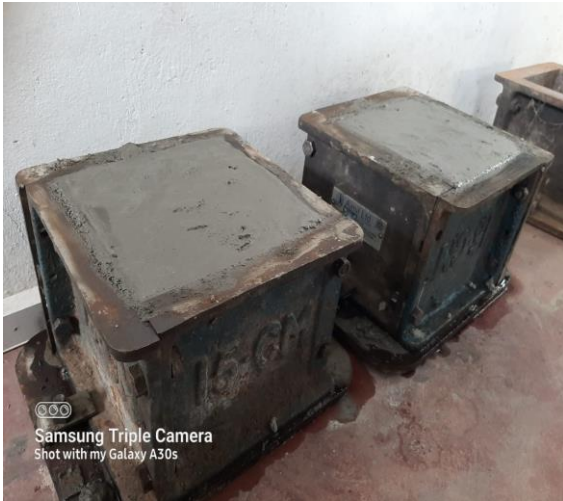
Fig 3:Cube moulds for compressive strength test
