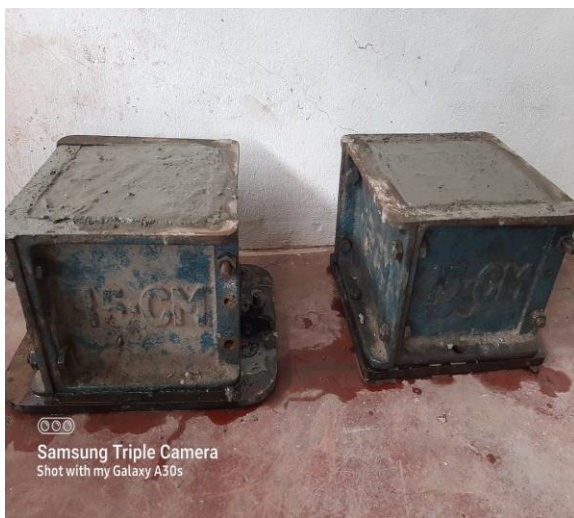
Fig 4:Cube moulds for compressive strength test
