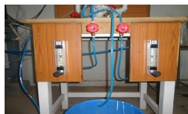
Fig. 1. Purge Rotameters for hot water and cold water flow measurement
