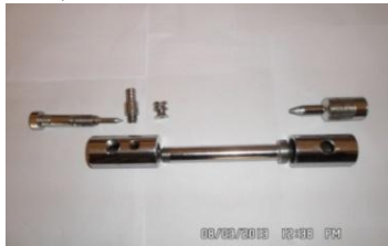
Fig 3 Components of modified vortex tube used for experimentation
