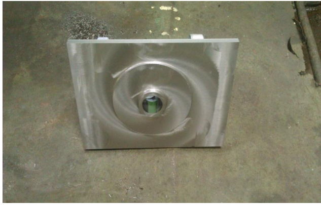
Fig. 6. Complete geometry of Radial Drill Head Feed Box Housing
