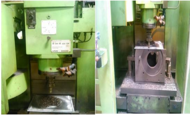
Fig. 4. Setup and machining of Radial Drill Head Feed Box Housing
