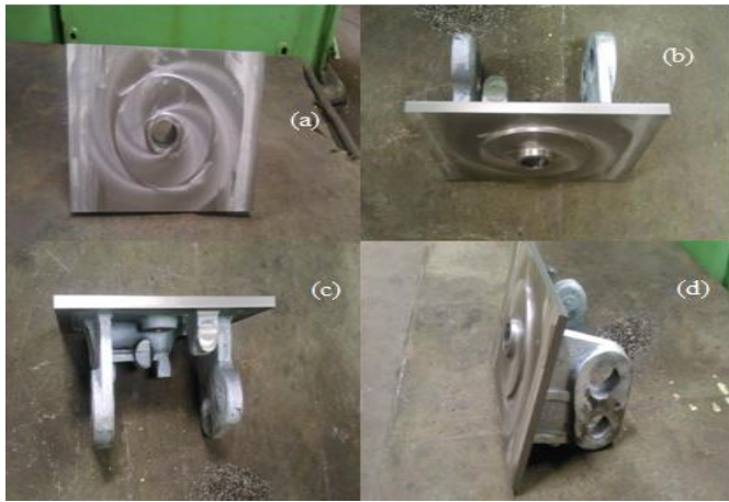
Fig. 7. (a) Front View (b) Top View (c) Back View (d) Side View of Radial Drill Head Feed Box Housing
