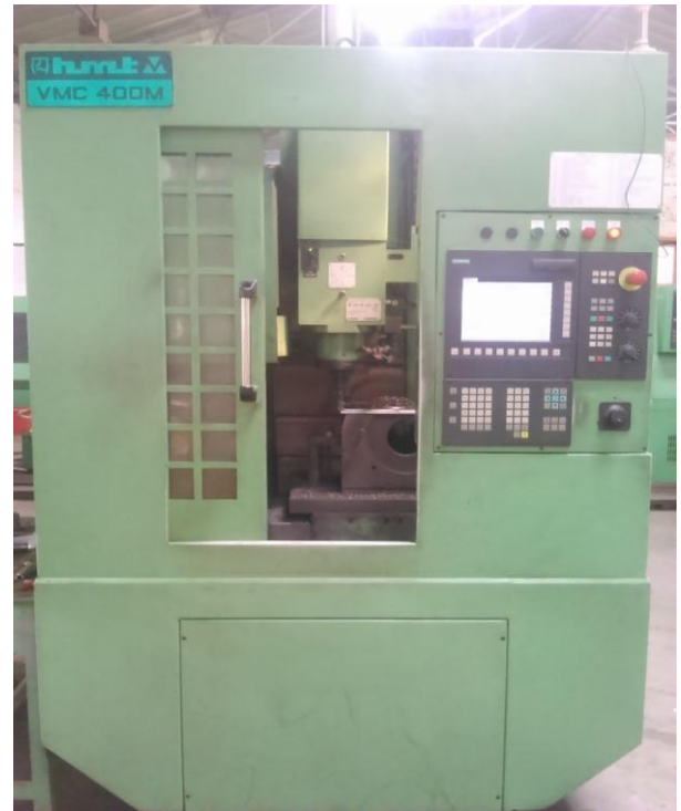
Fig. 2. Vertical Machining Center (VMC 400)
