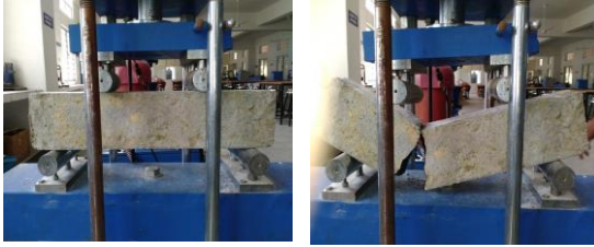
Fig. 4 Flexural strength test
