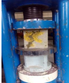
Fig. 2 Compressive strength test
