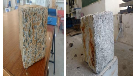
Fig. 5 Acid attack on cubes
