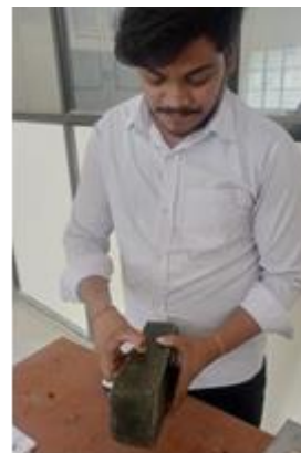
(No Scratch of plastic brick so brick is hard)
