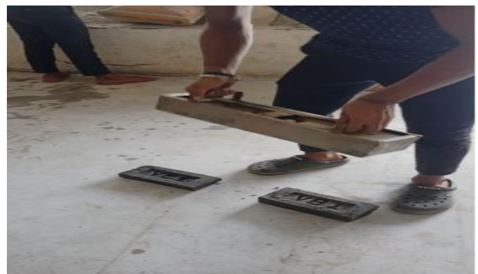
Moulding of Plastic Brick De-Moulding of Plastic Brick
