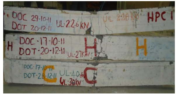
Comparison of Hooked End & Crimped Fibre RC Beam with Conventional RC Beam
