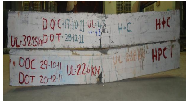
Comparison of Hybrid Fibre RC Beam with Conventional RC Beam
