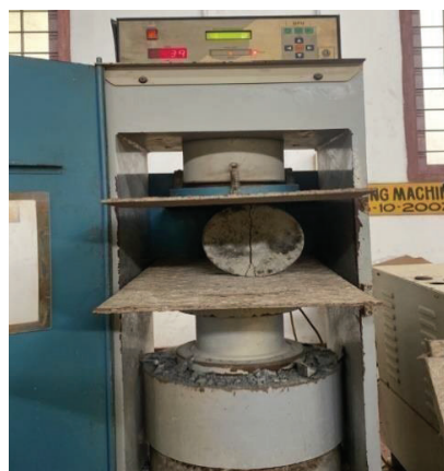
Fig 4.4 Split tensile strength test
