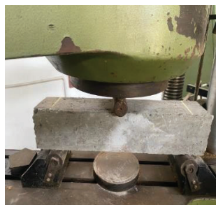
Fig 4.5 Flexural strength test
