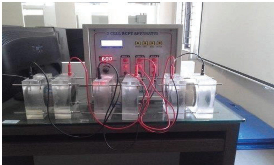
Fig. 3.16 Rapid Chloride Penetration Testing of specimen
