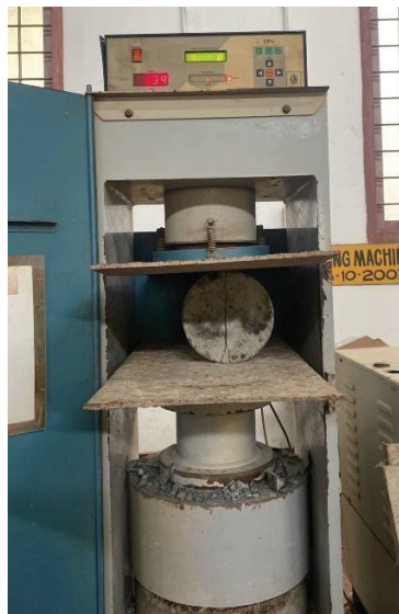
Fig. 3.15 Split tensile strength testing of specimen (Source: by author)
