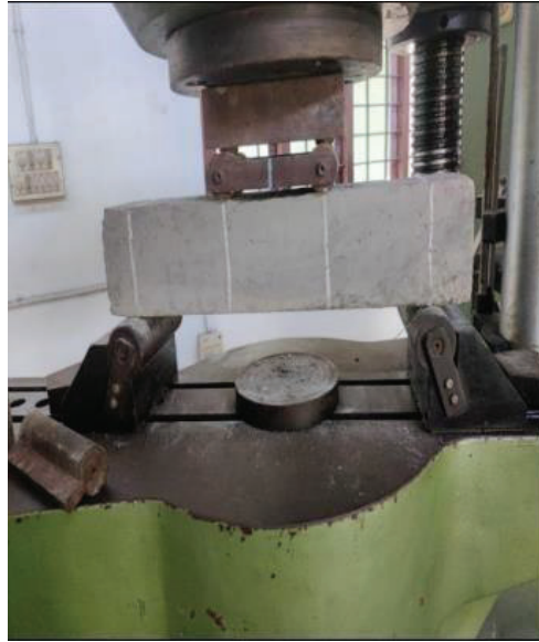
Fig 3.14 Flexural strength testing of specimen (Source: by author)
