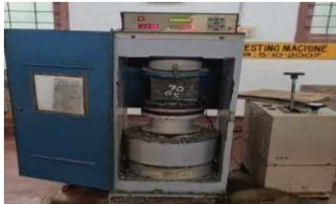
Fig 3.13 Compressive strength testing of specimen
