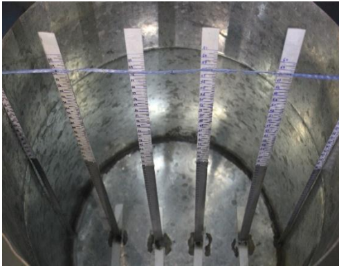
Fig. 7. Experimental set up for measurement of sloshing wave height
