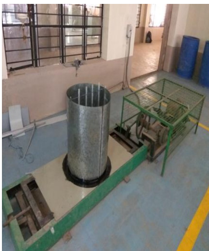
Fig. 4. Water Tank attached to Shaking Table
