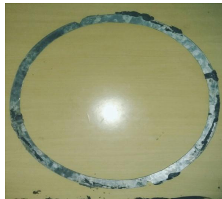
Fig. 5. Horizontal Ring Baffle Wall
