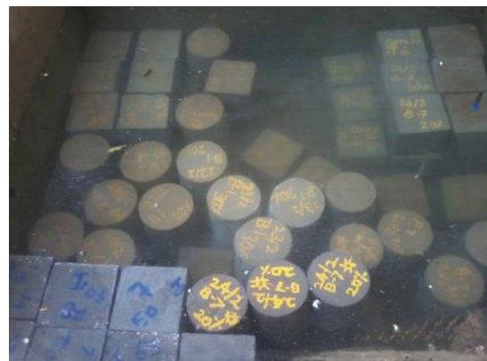
Fig 5 Curing of specimens
