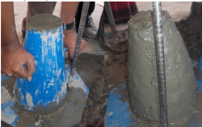
Fig 2 Slump Cone Test
