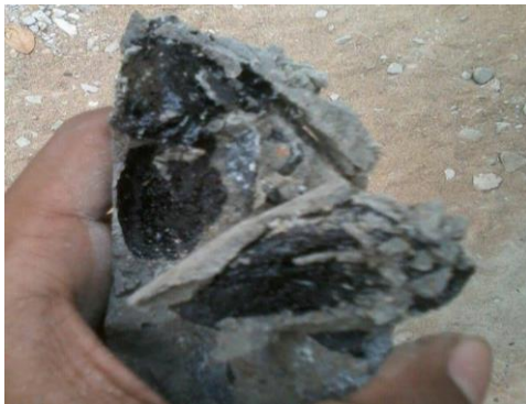
Fig 11 BCA in Concrete After Failure
