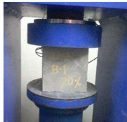
Fig 9 Testing of Specimen in UTM
