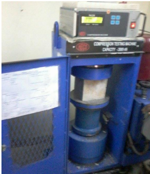
Fig 6 Compression Test Machine (CTM)
