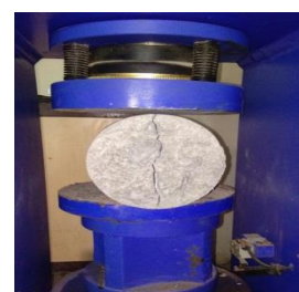
Fig 5: Split tensile strength test
