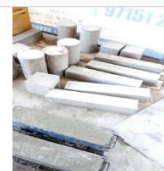
FIGURE.5.5 – Cylinder Casted for determining Tensile Strength
