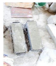
FIGURE.5.7 – Prism Casted for determining Flexural Strength
