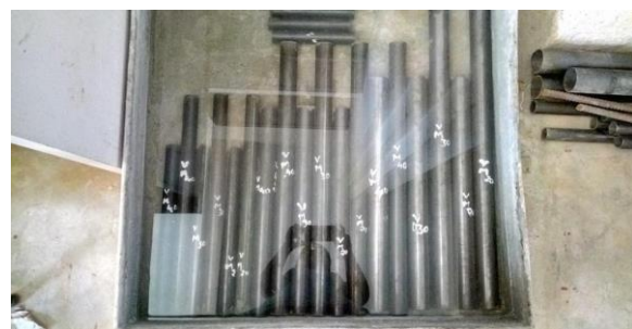
Curing of specimens
