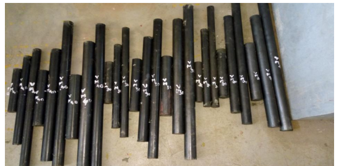
Specimens filled with different grade of SCC
