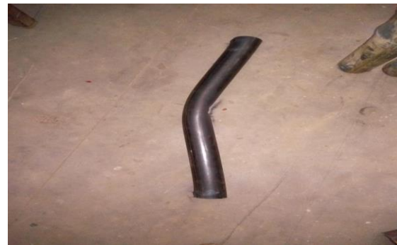
local buckling in the hollow steel tube on loading
