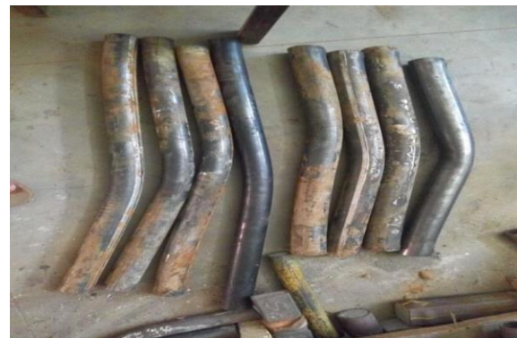
Buckling of the concrete filled and hollow steel tubes
