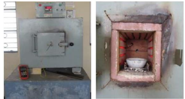
Fig.1. Muffle furnace, Heating of SiCat 700° C
