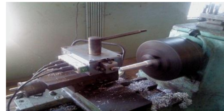
Fig :4 Turning operation of Al-Cu-SiC work piece with force dynamometer
