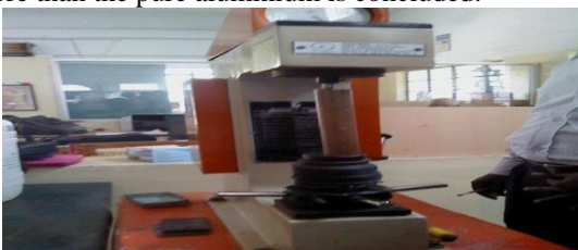
Fig :3Brinell hardness test for Al-Cu-SiC
