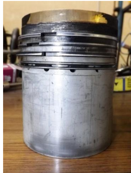
Fig. 2 Photo Graphic View of Aluminium Piston with Brass Crown and Air Insulation
