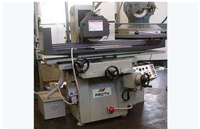
Surface Grinder with electromagnetic chuck, inset shows a Manual magnetic chuck
