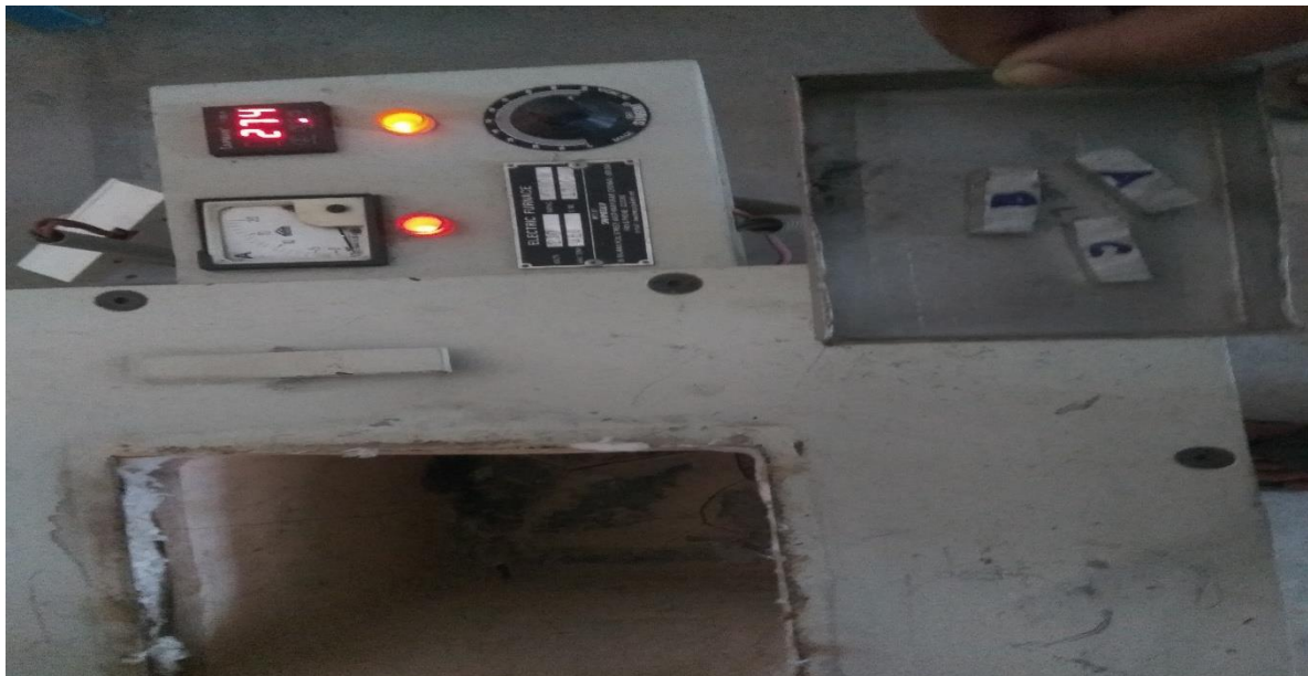
Fig 10 Induction furnace at constant temperature for 3 hours.
