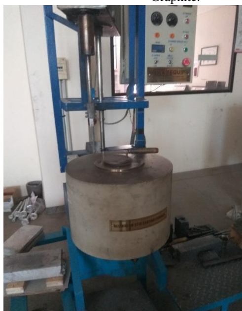
Fig 1 STIR CASTING PROCESS SETUP
