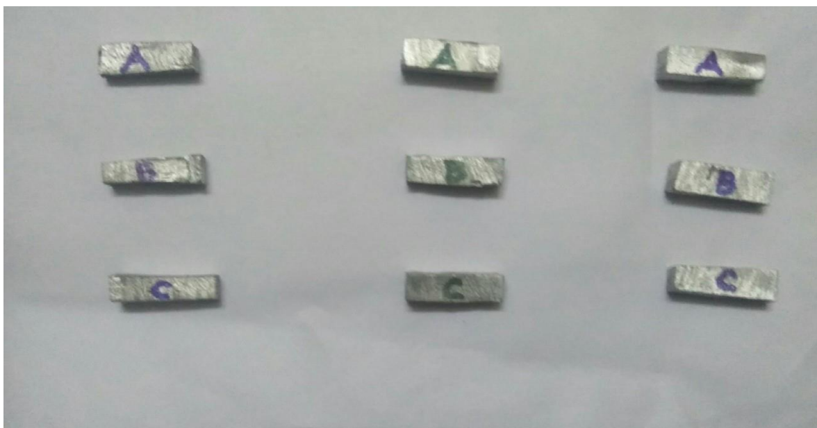
Fig 3 Sample specimen 8 mm x 8 mm of cross section
