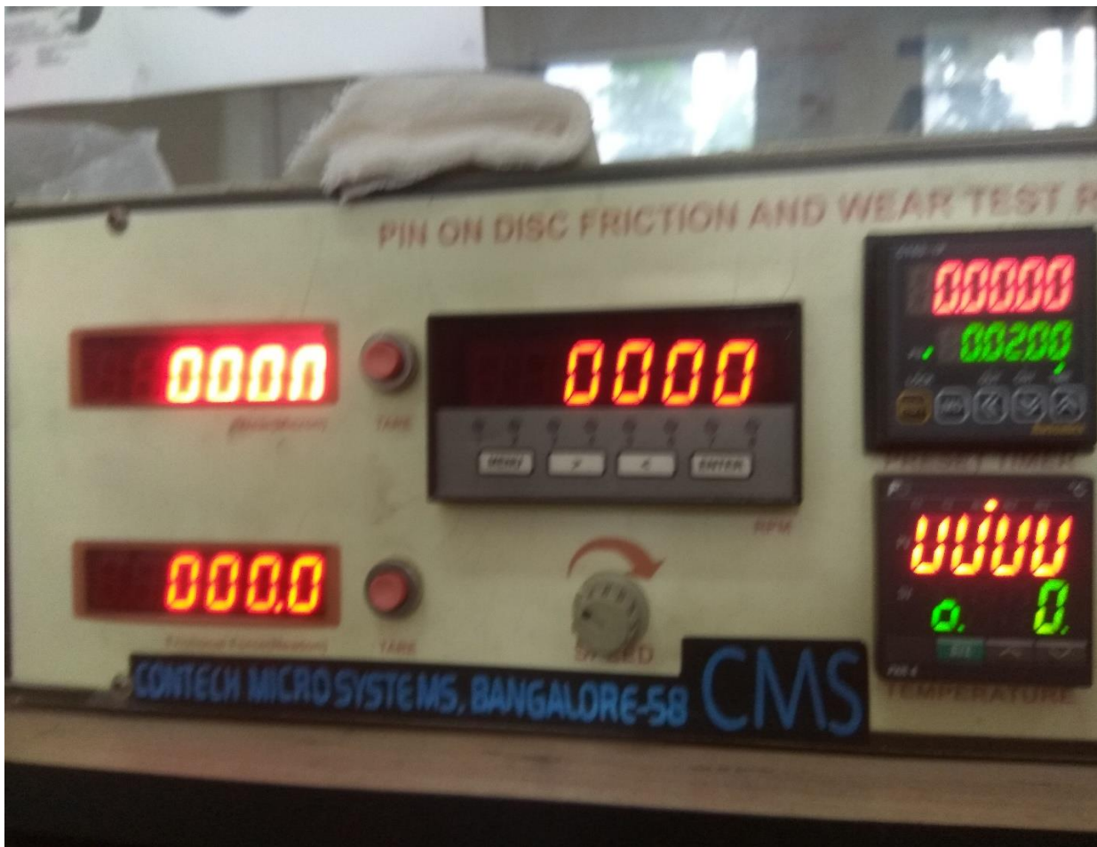
Fig 5 Wear test instrument at start position
