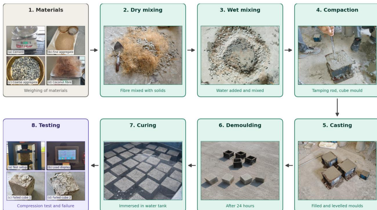
Fig. 1. Flowchart of the experimental procedure and the materials used for testing
